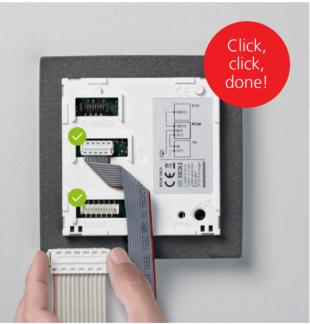
Only a few terminal blocks are needed for rapid installation of the complete system. The stable mounting frame accommodates the modules. The optional anti-theft protection can also be housed here.
